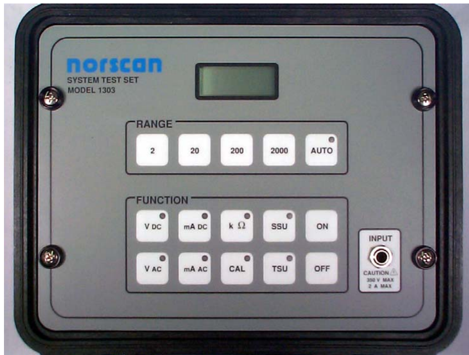
Figure 1: 1303 System Test Set – top view
