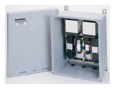
The 51300 Termination Protection Assembly (TPA) is installed at a building location where cable locate and/or monitoring terminations are required. The 51300 is used at the cable of origin in the cable vault or at the building entry point to safely terminate a fiber optic cable armor. locate wire or copper pair conductor. The assembly is pre-wired in an enclosure to allow for easy installation at the building entry location.
