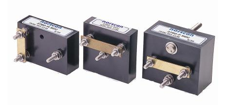
The 2785 Sheath Grounding Unit (SGU) connects to the cable armors and provides a low impedance ground path for high voltage transients while allowing tone location and monitoring signals to pass. The 2785 SGU is designed to fit into standard 3 inch or larger pedestals, marker posts and Big Fink<sup>™</sup> test stations. The 2785 SGU is environmentally sealed in a field rugged UV resistant case. A bond bar opens for east/west isolation and testing while still providing full surge protection.
